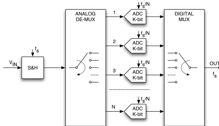
Time-interleaved ( $TI$ ) technique ( $z \rightarrow z^M$ ) is attractive for  $\Sigma\Delta$  as the  $OSR$  increases without speeding-up analog blocks.
