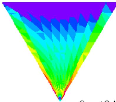
Current at First Resonance Reaches to the Top of Bowtie Antenna
