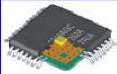
Visualization of antenna (the brown layer) integrated on a package substrate
