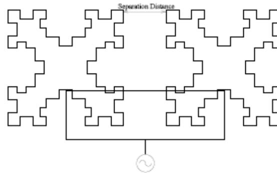
Thin Feeding Network for Fractal Array Elements
